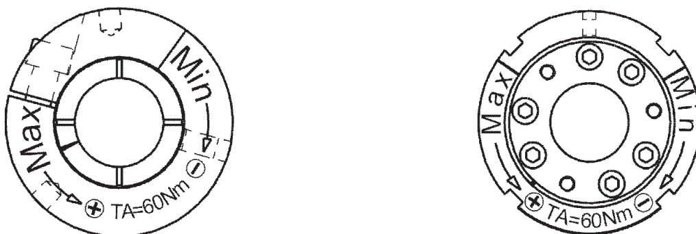
Marking of torque limiter after delivery (left: clamping hub; right: adjustment nut)
